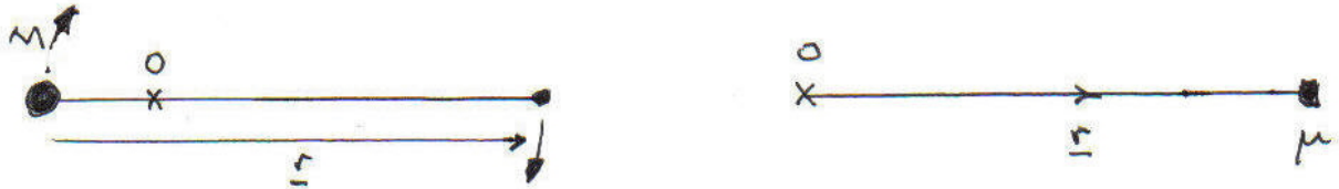
Figure 59: Equivalent system: reduced mass
