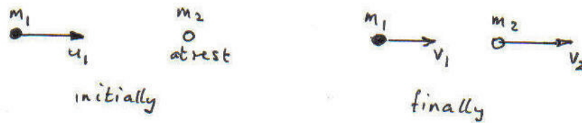
Figure 36: Head-on elastic collision
