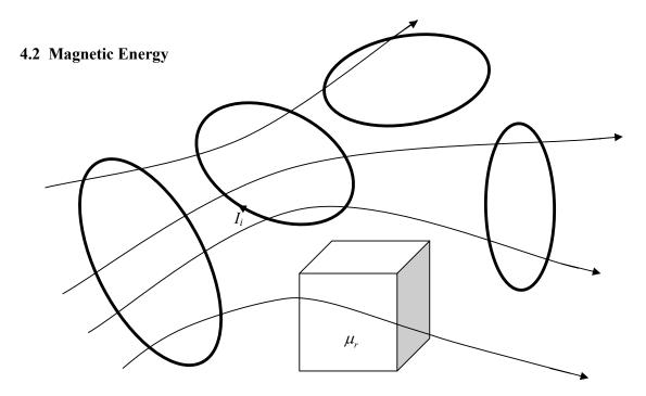
This argument looks very artificial but is actually quite general We consider an isolated region containing a number *n* of fixed electric circuits. The *i*th circuit has a battery which is supplying a slowly varying current  $I_i(t)$  and the circuit is threaded by a flux  $\Phi_i(t)$  due to the combined effect of all the circuits and of fixed pieces of magnetisable material in the region. For the purposes of argument we ignore ohmic losses in the circuits with steady currents.
