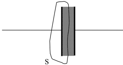
We can calculate the flux of  $\mathbf{E}$  through a Gaussian surface  $S$  like a sealed bag completely enclosing one plate but cutting through the dielectric. Assuming  $\mathbf{E}$  is only significant inside the capacitor, and is uniform and perpendicular to the plates, then from (1.9)
