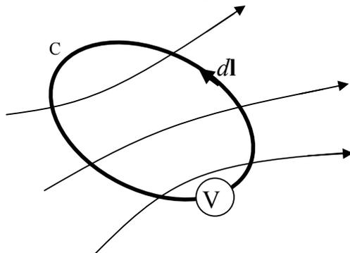
A conducting circuit  $C$  may be intersected by a  $\mathbf{B}$  field which gives a flux
