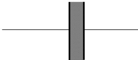
then for the same voltage  $V$  across the plates we can store more charge  $Q$ . (N.B. this subject needs so many symbols that we can never completely avoid re-using them, like  $V$  for volume and  $V$  for volts.) That means that the capacitance  $C = Q/V$  goes up when the dielectric is inserted. We call the dimensionless factor by which it increases the dielectric constant  $\kappa$ . The formula relating capacitance to gap spacing  $d$  and plate area  $A$ , in vacuum, is
